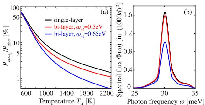
**Figure 4.** (a) Fraction of below-band-gap heat exchange for the same results as those in Figure 3 for an applied bias of  $V = V_{\text{oc}}$ . (b) Below-band gap normalized emission spectrum,  $\Phi(\omega)$ , near the Reststrahlen band of InAs. The black curve corresponds to the single-layer emitter case, while the blue and red ones correspond to the bilayer emitter with  $\omega_{p2} = 0.5$  and  $0.65$  eV, respectively.
