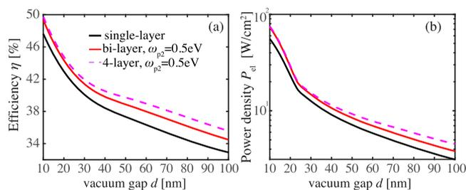
**Figure 5.** (a) Efficiency and (b) power density as a function of the vacuum gap size for the single-layer emitter case with  $\omega_{p1} = 0.44$  eV, the bilayer case with  $\omega_{p2} = 0.5$  eV, and the four-layer case with  $\omega_{p3} = 0.6$  eV and  $\omega_{p4} = 0.575$  eV, as in Figure 2.
